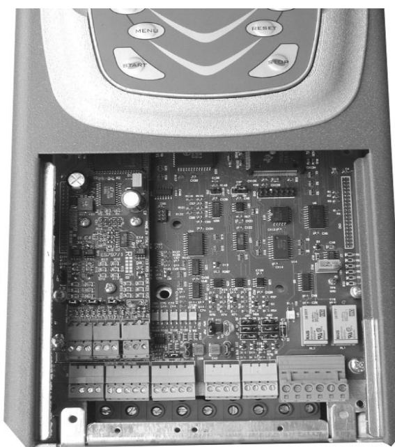
Fig. 4.12 Encoder board fastened to its slot
