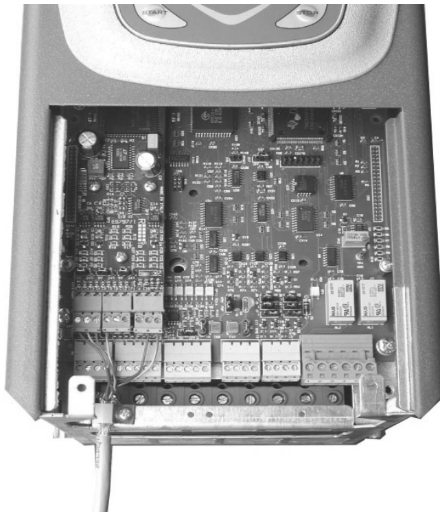
Fig.4.18 – Wiring the encoder cable
