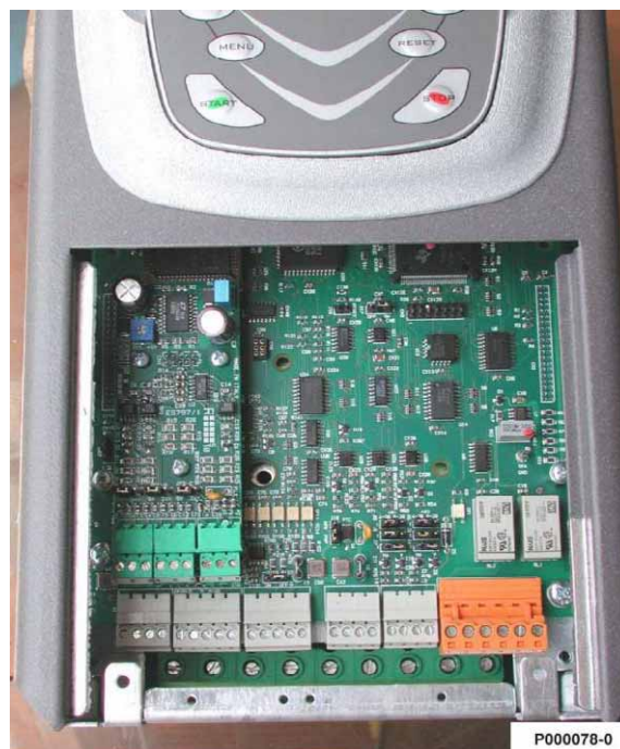
Figure 3: Encoder board fastened to its slot
