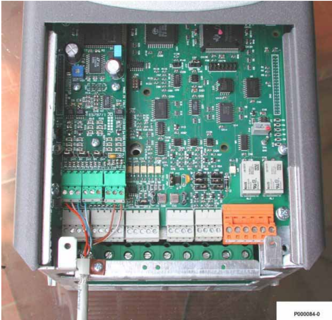
Figure 9: Wiring the encoder cable
