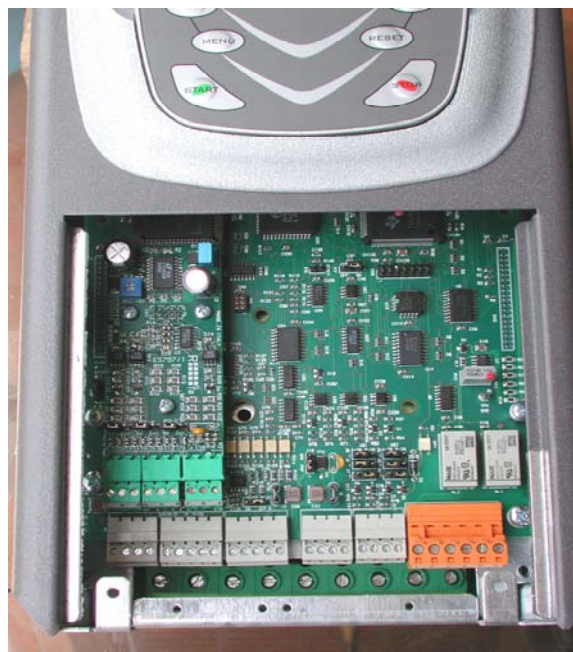
Fig.4.13. Encoder board fastened to its slot
