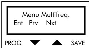
Press PROG (Ent) to access the first page of the Multifrequency submenu. Press ↑ (Nxt) and ↓ (Prv) to scroll through the submenus.
